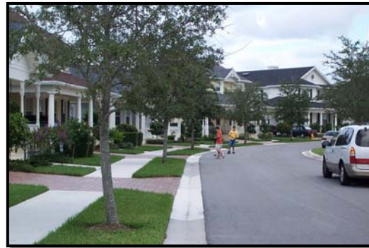
The Colony Design Guidelines emphasize safe, pedestrian-friendly residential development and streetscapes. In this photo, the setback from curb to front porch is generous enough to allow a double row of trees. Homes with "eyes on the street" and generous parkways with mature street trees provide a safe pedestrian atmosphere and add an attractive, unifying visual element.
